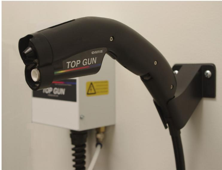
All functionality is built into the gun, including a flow control valve for adjusting the airflow, a balance adjustment for calibration, and a two-level LED. The air gun has a filter at its exit to ensure that out-flowing air is clean.
