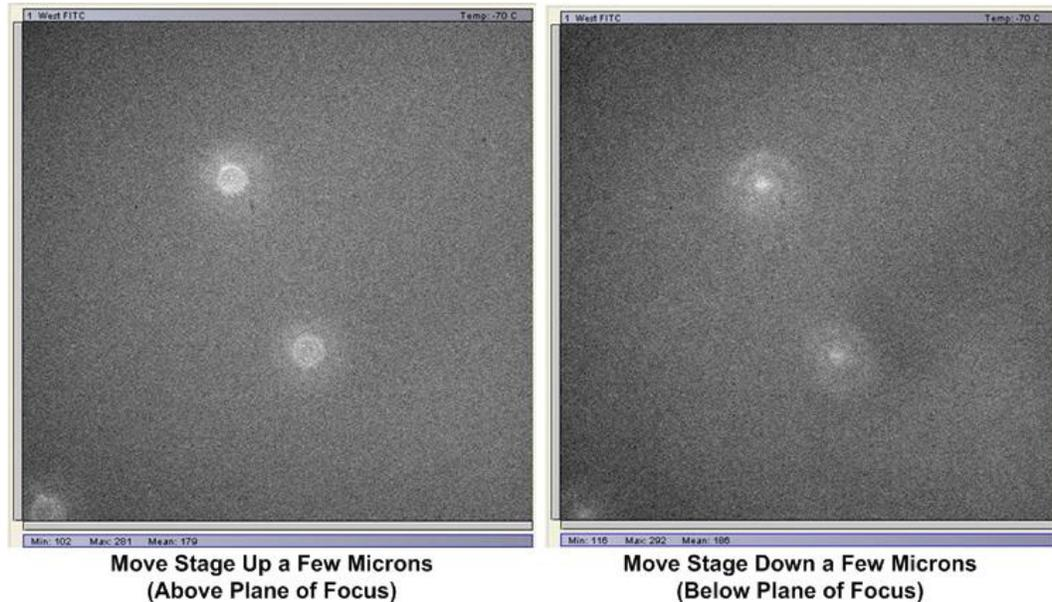
6. Repeat Steps 4 and 5 until spherical aberration is minimized.
