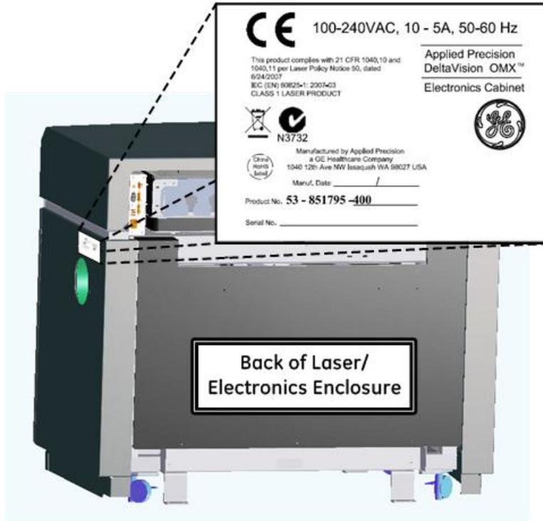
The following CE label (4 X 2.88"), containing specific system information, is attached to the back of the Microscope Enclosure cabinet (as shown).
